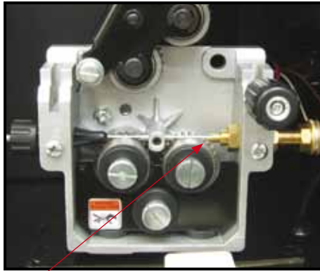
(5) Feed the wire through the drive roller and into the outlet guide tube of the wire feeder.
