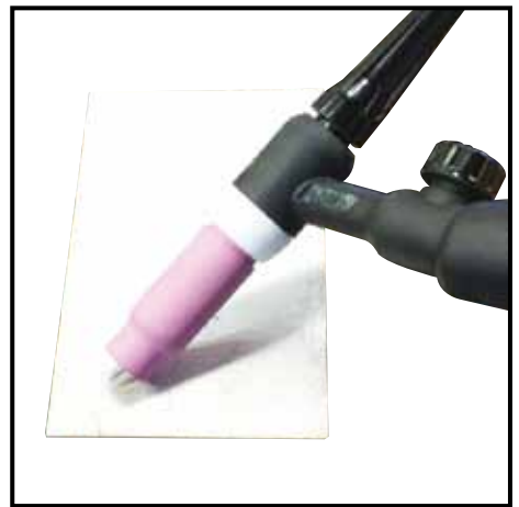
(7) Lay the outside edge of the Gas Cup on the work piece with the Tungsten Electrode 1- 2mm from the work piece.
