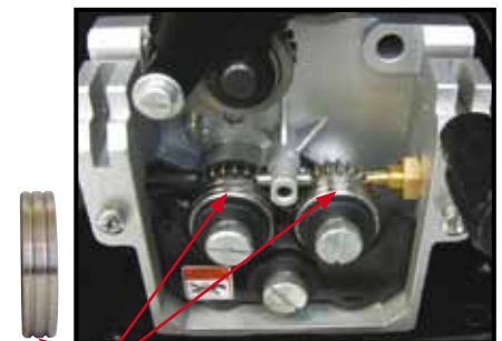
(9) Install a U groove drive roller of the correct size for the diameter wire being used.
