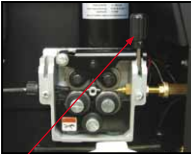
(9) Close down the top roller bracket and clip the pressure arm into place. Apply a medium amount of pressure to the drive roller
