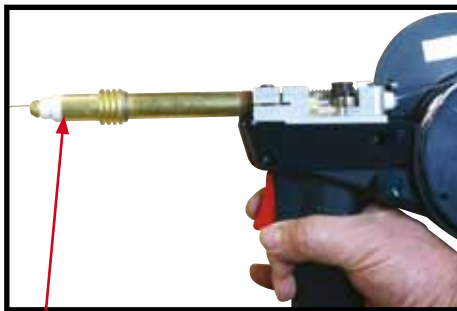
(12) Remove the gas nozzle and contact tip. Pull the trigger to drive the wire through the neck until it exits the contact tip holder
