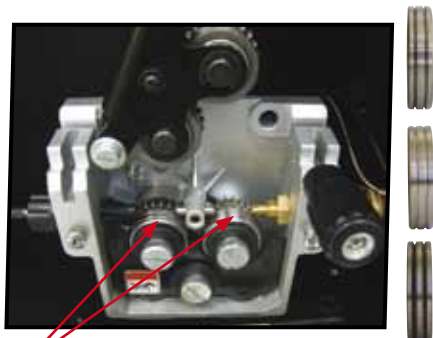
(6) Fit the correct type and size of drive rollers.V Groove for Hard Wires. U Groove for Aluminium. Knurled for Flux Cored
